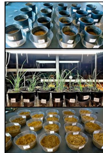
Fig 1.Placing plastic containers used for leachate collection atop pots with polluted soils treated with the various organic treatments but without switchgrass, (Middle): Switchgrass growing in vegetated pots in a lab with 24-hour lighting, (Bottom): After the experiment, soil from the pots was taken for analysis.
