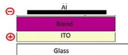
Fig. 4 Typical cell Structure of Organic OSC
