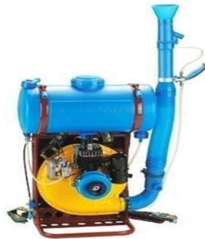
Fig. 2.2.2.2. Motorized Knapsack Mist-blower cum Duster
