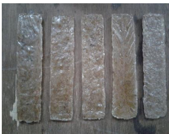
(b) Jute-Epoxy specimen
