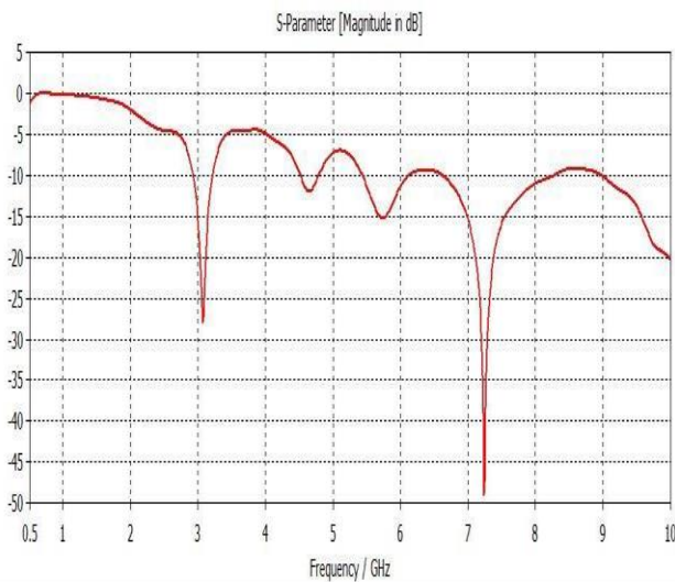
Fig 6 S parameter plot after the introduction of notch
