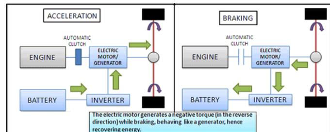
Whenever the motor runs in one direction the electric energy gets converted into mechanical energy, which is used to accelerate the vehicle. But when the motor runs in opposite direction it functions as a generator, converts mechanical energy into electrical energy, making it possible to utilize the driving axle to turn the vehicle, which regenerates electric energy for storage. This energy can be used for recharging the battery.
