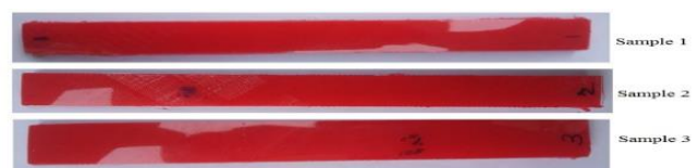
Fig3.5 3D Printed Flexural Specimens
