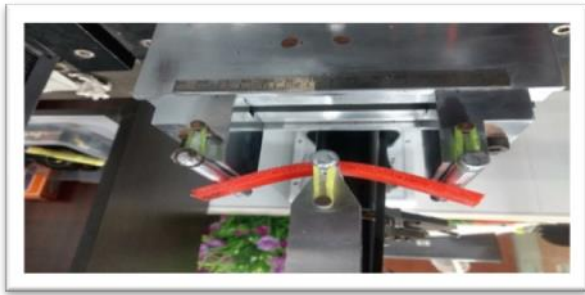
Fig 3.6 Process of Flexural Strength testing
