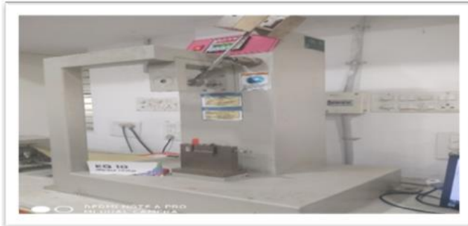
Fig4.7 Izod Impact Testing Machine
