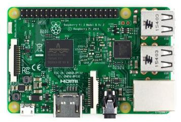
Whilst maintaining the popular board format the Raspberry Pi 3 Model B brings you a more powerful processer, 10x faster than the first generation Raspberry Pi. Additionally it adds wireless LAN & Bluetooth connectivity making it the ideal solution for powerful connected designs.
