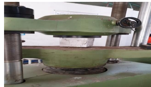
Fig 3.3 Testing of Compressive strength
