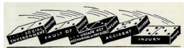
Fig.1:- Accident causation model
