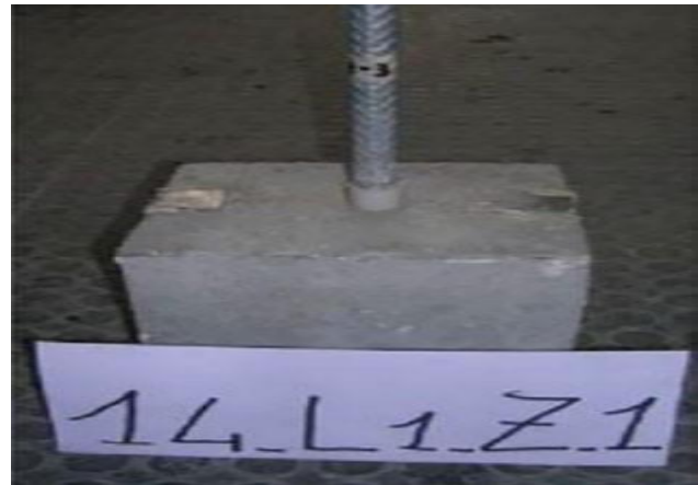
Figure 4. EPS LWC sample reinforced with zinc-coated steel bar. 34 (Reproduced from Ref. 34, with permission from Springer Nature.) [Color figure can be viewed at wileyonlinelibrary.com ]
