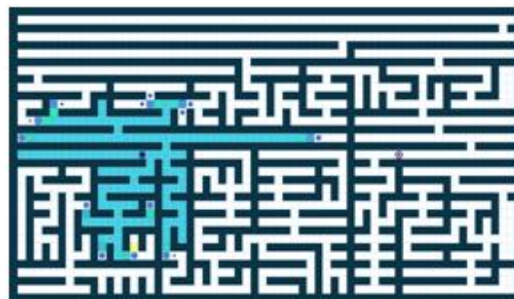
Fig. 1. Probing the grid space to find the most optimum path space (BFS)
