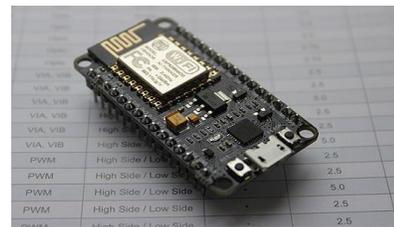
Fig.3.10: NodeMCU ESP8266 board
