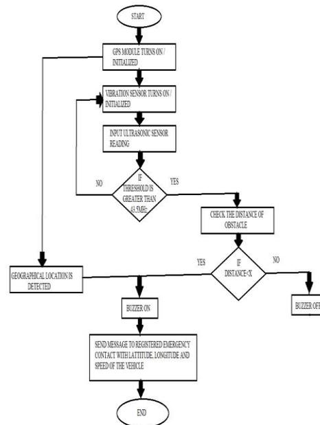
Fig.4.2: Flow diagram of VTV communication
