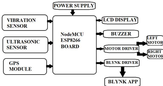
Fig.3.2: The proposed block diagram for vehicle-to-vehicle communication using IOT.
