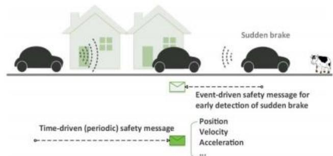
Fig.1.1: Collision avoidance using V2V communication
