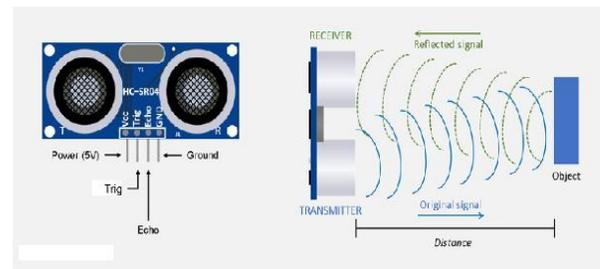
Fig.3.5: Ultrasonic sensor
