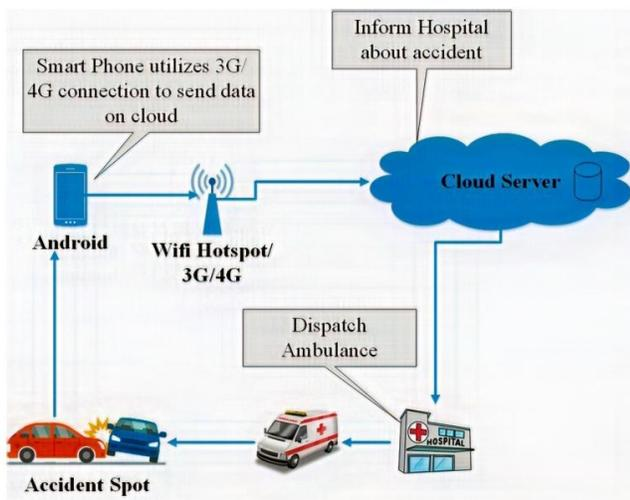
Fig.1.2: Accident Detection and Reporting System (ADRS)
