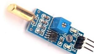
Fig.3.6: Vibration sensor
