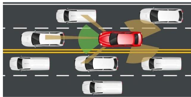
Fig.4.1: System scenario of V2V
