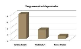
As you can see in above pictures it is specified that stiffness of bamboo is more than steel, also the energy consumed while construction is also less in bamboo material results in cost degradation of the project and more efficiency in work.
