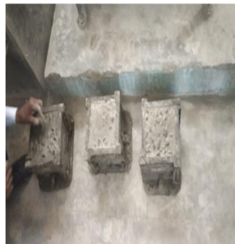
Photo No: 3 casting of cubes
