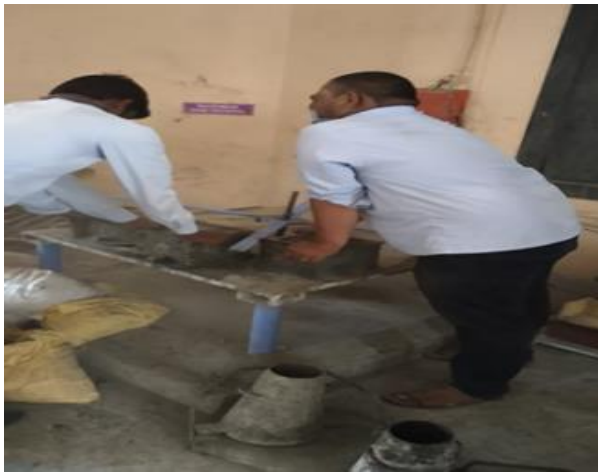
Photo. No: 4 Compaction of cubes using table vibrator
