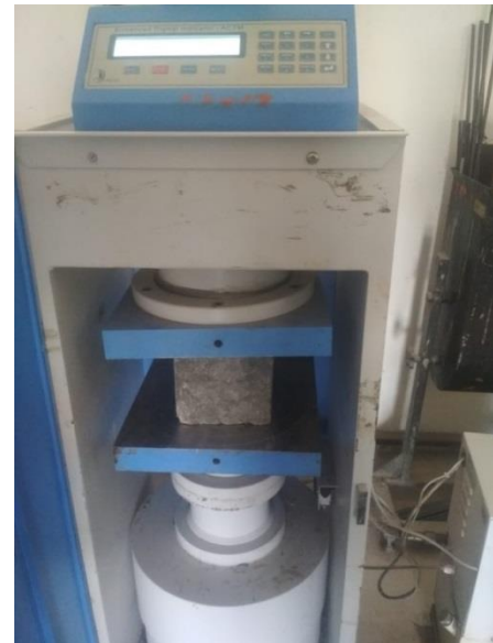
Fig1– Compressive Strength Testing (Universal Testing Machine)
