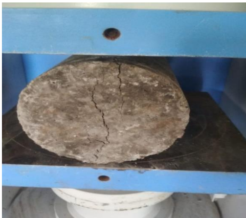
Fig5– Split Tensile Strength Testing (Universal Testing Machine)
