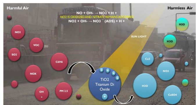
Figure 1- TiO 2 , Capturing energy from sun light to depollute the air- Photo catalytic Reaction
