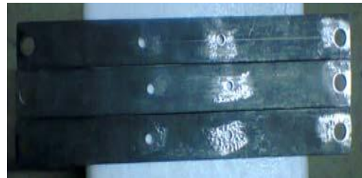
Fig.5: Holes drilled on links
