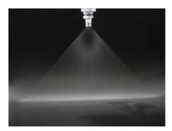
(i) To find jet nozzle velocity (V):  $\label{eq:Q} Q = AxV$
