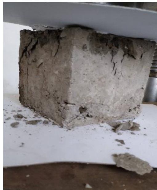
Figure 3.2 – Cube Specimen at time of Compressive Strength Test
