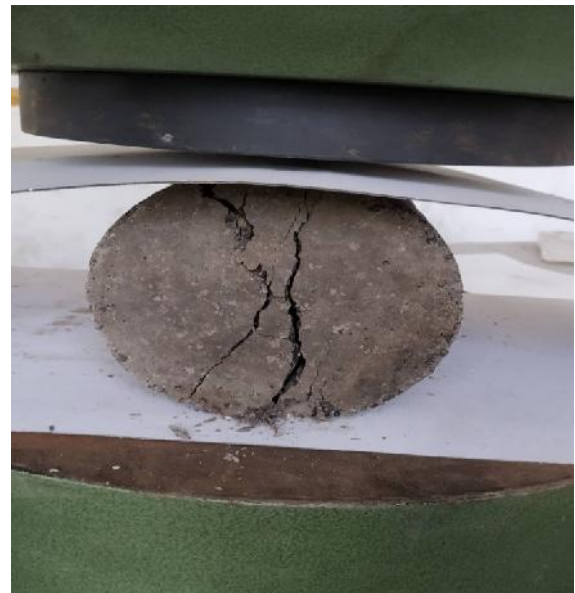
Figure 3.4 – Cylinder Specimen at time of Spilt Tensile Test
