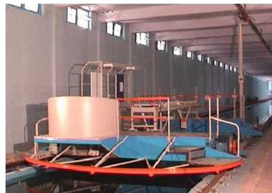
Fig .12.1 – Current Meter Rating Trolley
