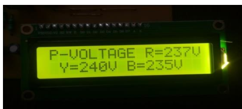
Figure11:- Phase Voltage Display On Lcd
