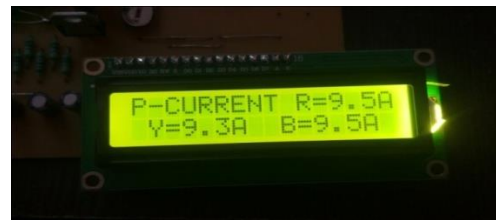
Figure12:- Phase Current Display On Lcd
