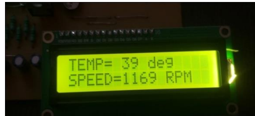
Figure13:- Temperature And Speed Display On Lcd
