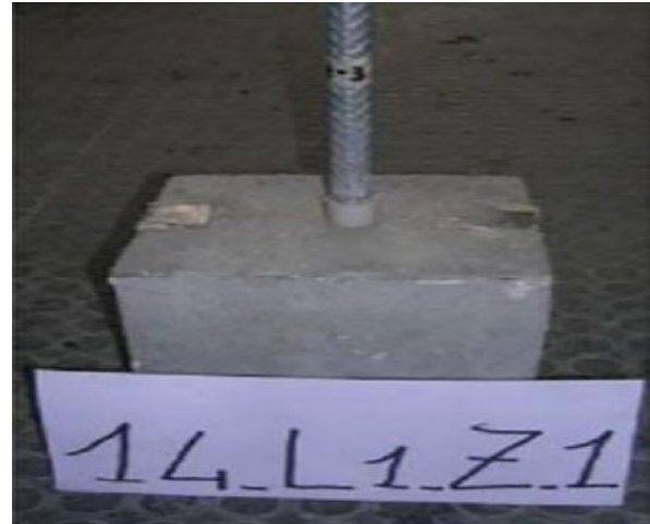
Figure 4. EPS LWC sample reinforced with zinc-coated steel bar 34 (Reproduced from Ref. 34, with permission from Springer Nature.) [Color figure can be viewed at wileyonlinelibrary.com ]
