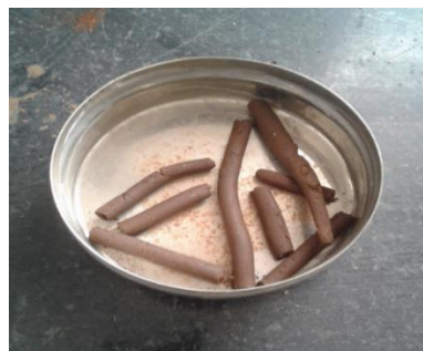
Fig : D Plastic limit (Soil Rolled in 3mm thread)
