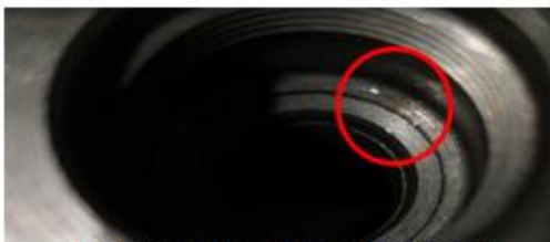
Fig 6. Dent indentations on Element seat
