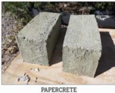
Fig. Casting the papercrete brick.
