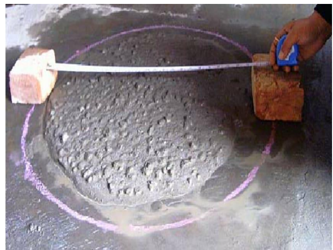
Fig.2: SLUMP TEST (Flow test),:T50
