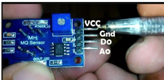
Fig2: Gas Sensor MQ2 Pinout
