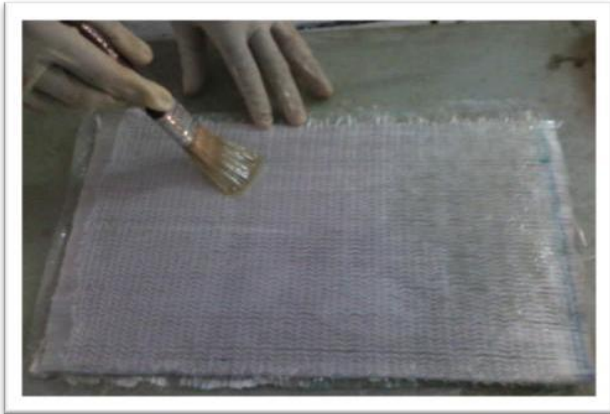
Fig. 7 Applying epoxy resin on fiber
