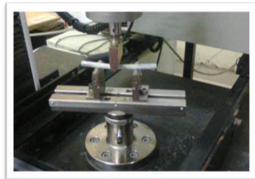
Fig. 12 During flexural test
