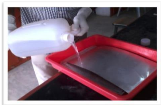
Fig. 3 Aluminium sheet cleaning with Acetone
