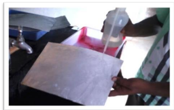
Fig. 4 Aluminium sheet cleaning with hot water
