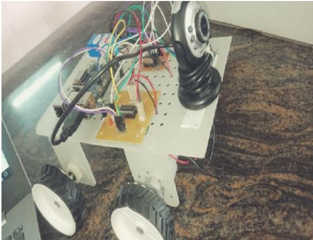
Figure 2 (a) constructional setup of proposed system
