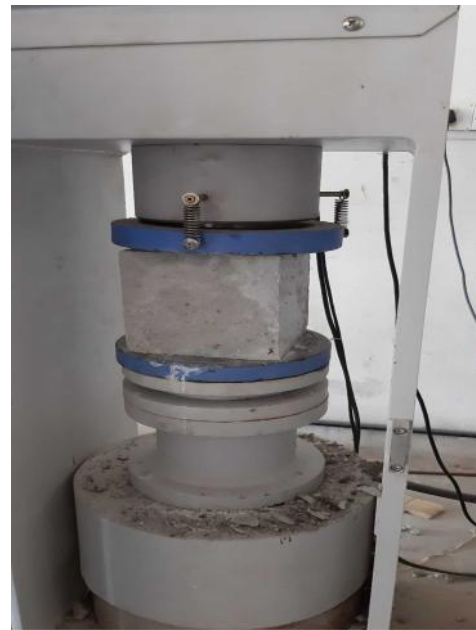
Fig. 3 Concrete Cubes tested in Compression Testing Machine
