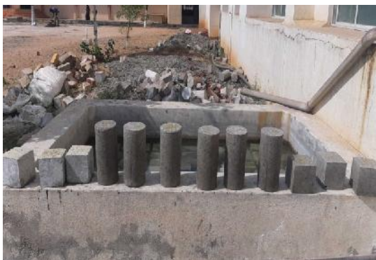
Fig.2 Cube and Cylinder Specimens after curing
