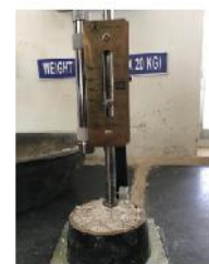
FIG.5.1.2. STANDARD CONSISTENCY TEST
