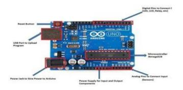
The Arduino Uno is a microcontroller board based on the ATmega328. The ATmega328 has 32 KB (with 0.5 KB occupied by the boot loader). It also has 2 KB of SRAM and 1 KB of EEPROM (which can be read and written with the EEPROM library). It has 20 digital input/output pins (of which 6 can be used as PWM outputs and 6 can be used as analog inputs), a USB connection (used to upload the programme), a power jack, an in- circuit system programming (ICSP) header, and a reset button.
