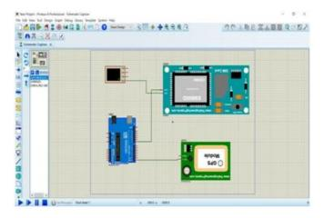
The vehicle tracking device is one of the best uses of the Arduino system. In the pandemic situation which we are facing today that COVID-19 best way to understand the vehicle tracking device is its simulation. For simulation we have used two software which are Arduino IDE and Proteus. Arduino IDE is well known to everyone. Well the Proteus Design Suite is a proprietary software tool suite used primarily for electronic design automation.
