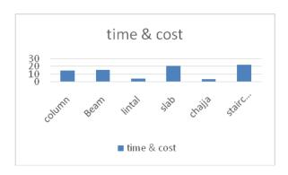
This graph shows that the components wise cost comparison in percentage. Column reduces 14.2%, Beam 15.433%, lintel 4.29%, Slab 20.8%, lintels with Chajja 3.66% and Staircase 21.78%.
