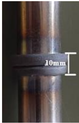
Figure 3 Typical flash showing burn-off length
