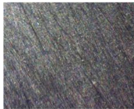
Figure 8 Macrograph of pitting corrosion tested joint
