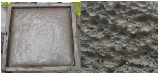
Fig. 2 a) Casted Aerated Concrete b) Pores present in casted AAC blocks
