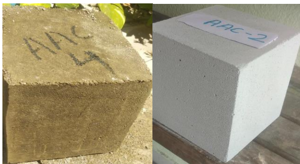
Fig. 3 Casted aerated blocks before and after autoclaving process
