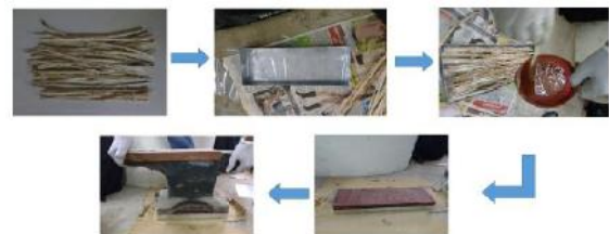
Fig.3. Flowchart for fabrication process
