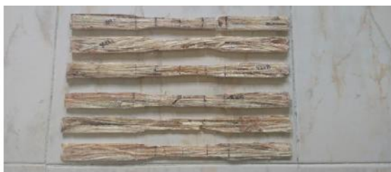
Fig.5. Specimen after tensile test
