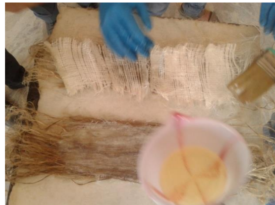
Figure 3.1 Okra-Epoxy Composite Specimen Preparation
