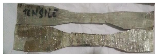
Figure 4.1 Tensile test specimens
