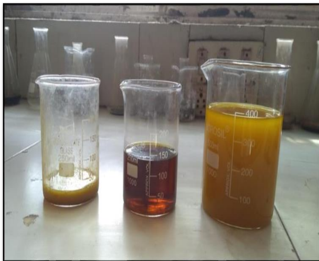
Fig. No. 6: By products of transesterification reaction after separation
