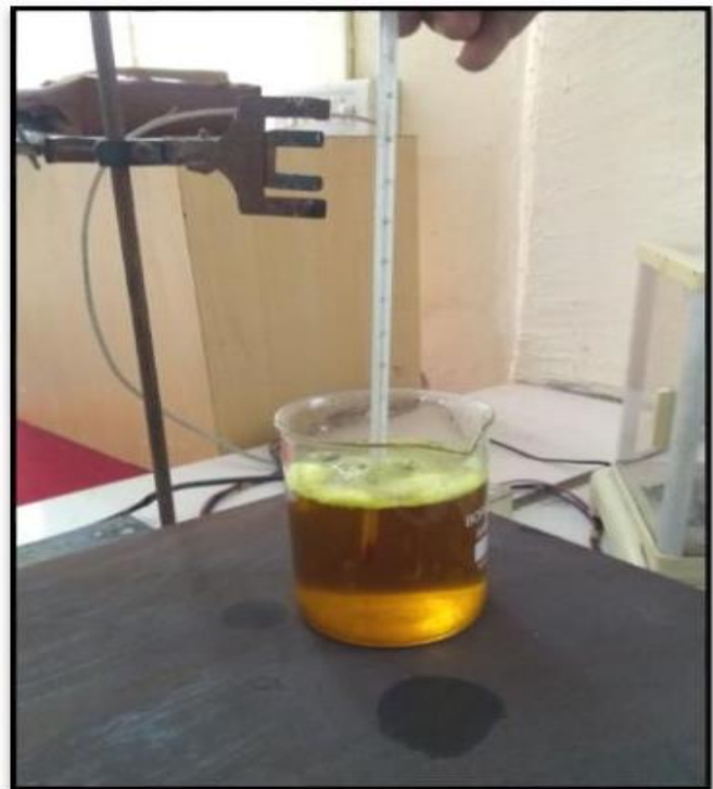
Fig. No. 7: Biodiesel after heating at 100°C
