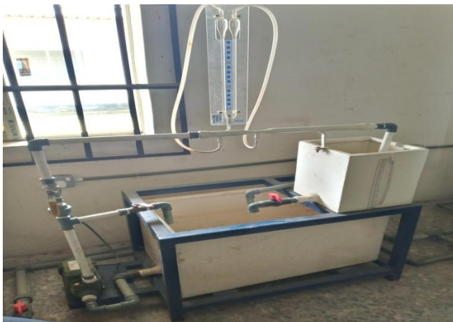
Figure 1.2: Shows the manufactured Venturimeter flow rig being integrated alongside other fluid mechanics equipment in the fluid mechanics laboratory
