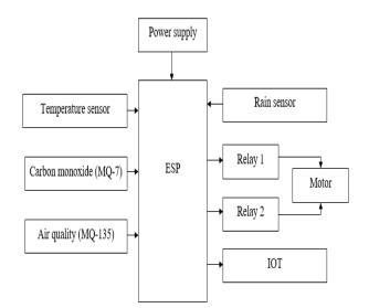
In this system, the hardware components are power supply, ESP32 microcontroller with WIFI module, temperature sensor LM35, carbon monoxide sensor MQ7, air quality sensor MQ135, rain sensor, relays, buzzer and dc motor. The software components are Arduino-IDE and embedded C.
