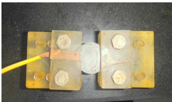
Fig.6. EMM Micro holes on plate.
