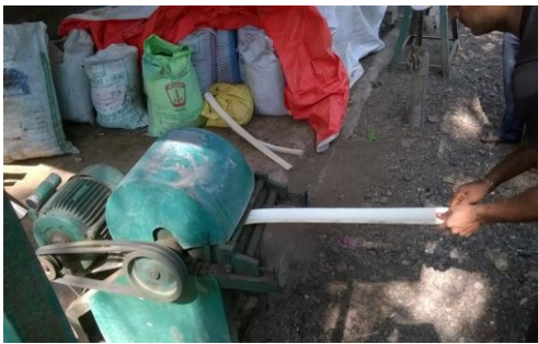
Figure 1.2.1 Process of Manufacturing of Banana Fibre
