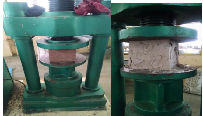
Fig 4.2 Testing of cubes for compressive strength
