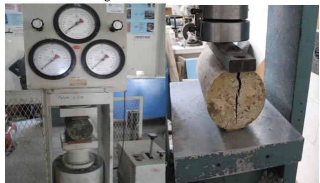
Fig 4.3: testing of specimens for split tensile strength
