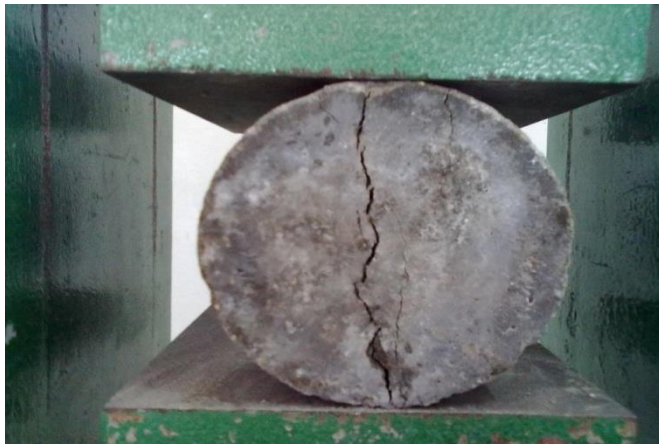
FIG. 1.4 Testing of cylinders for Split Tensile Strength
