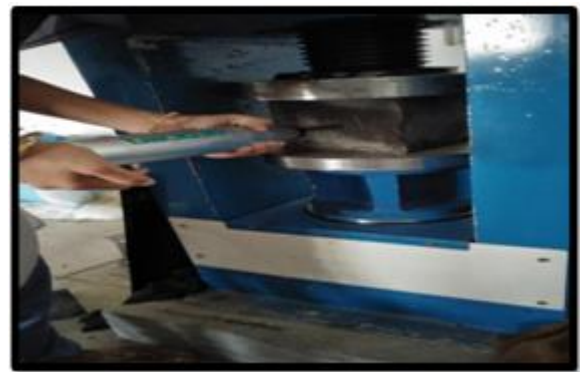
Fig2: Conducting Rebound hammer test
