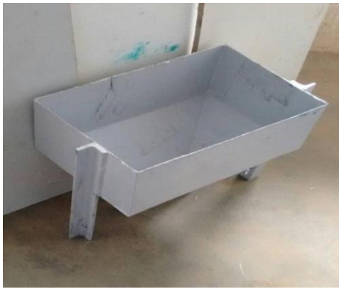
Fig.24 Seed hopper after fabrication
