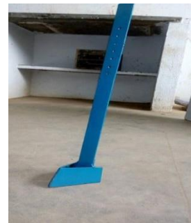
Fig.27 Furrow opener after fabrication
