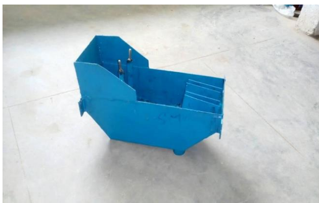
Fig.20 Seed metering container after fabrication
