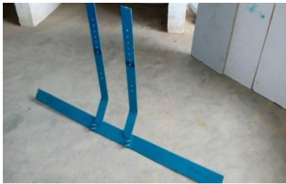
Fig.13 Leveler blade after fabrication
