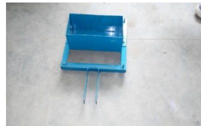
Fig.10 Weedicide container with weeder frame after fabrication
