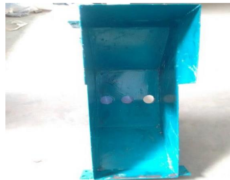
Fig.22 Fertilizer metering container after fabrication
