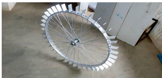
Fig.15 Spike wheel after fabrication
