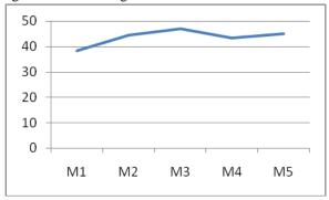
The above results indicate that the flexural strength of the concrete is maximum in 30% steel slag replace with coarse aggregate . The variation of steel slag replace with coarse and fine aggregate is shown in figure 5.2.
