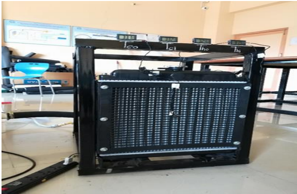
Fig.4.1.1 Radiator with cooling fan
