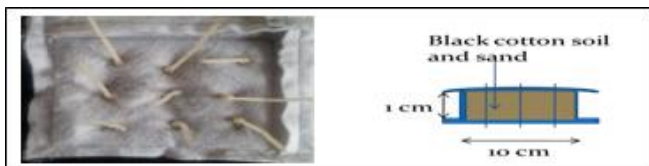
Fig.3.3(c) Filling Soil Mixture and Stitching Geotextile on Top
